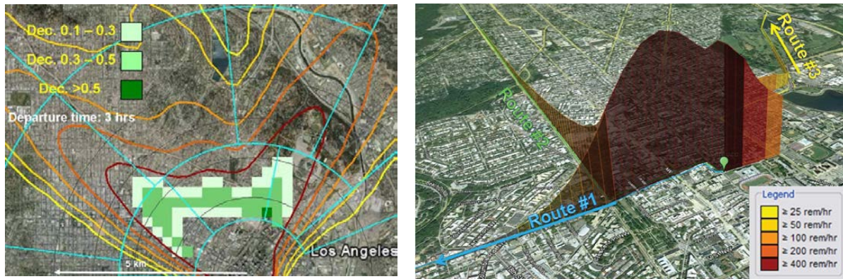
Figure 8: Examples of Nuclear Evacuation Analysis Code Analysis Outputs. Left: Example of Three Potential Evacuation Routes with an Overlay of Time-Dependent Radiation Exposure Resulting from Use of Each Route. Right: Analysis of the Decrease in Fatality Probability Afforded by a Departure 3 Hours Later Than the Reference Strategy. (From Sandia National Laboratories)
