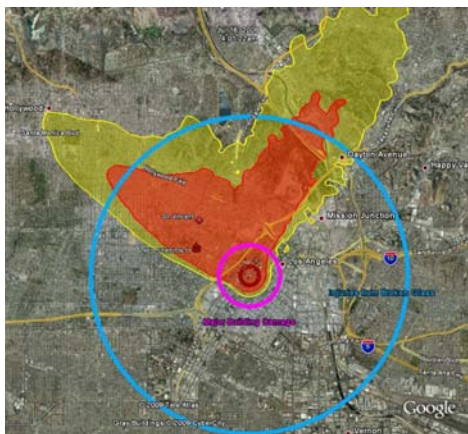
Figure 29. Areas of acute effects from blast (blue) and fallout (yellow, orange) for Los Angeles Scenario.
