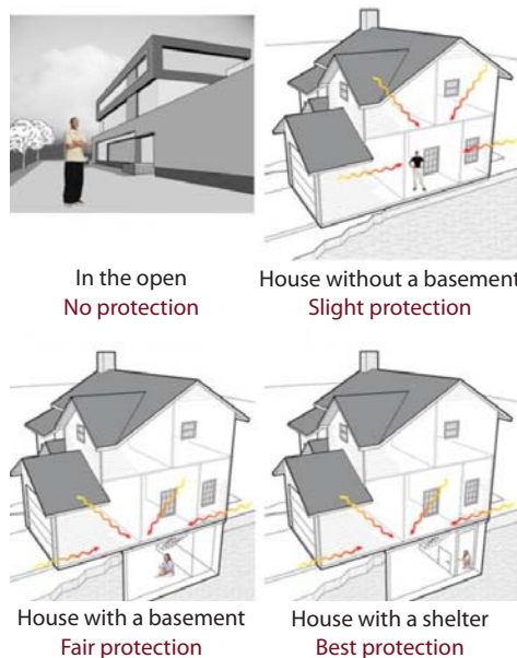
Figure 3. Protection can vary depending on its location in the building.
